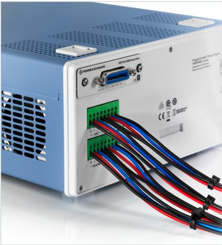
Backplane of an R&S®HMP4040 with force and sense connections.
