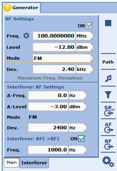
Frequency modulation with an integrated interfering signal
